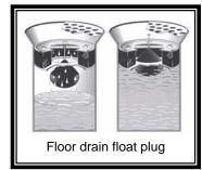
**Precautions:** A plug left in the floor drain may contribute to a wet basement if water from a laundry tub spill or a leaky pipe cannot drain out. Float plugs are known to have been jammed open by a small amount of debris. A plug does not tell you if there is a problem in your sewer service line. If the plug is not tight enough, pressure can eject it. Therefore, a plug is not recommended for flood depths greater than one foot.
